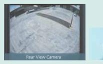
A rear view camera is installed as standard to simplify checking for safety behind the machine. The picture appears on the color monitor.
