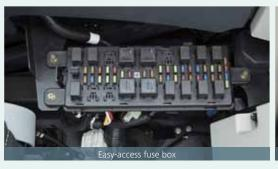
More finely differentiated fuses make it easier to locate malfunctions.
