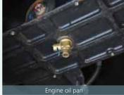
Engine oil pan equipped with drain valve.
