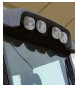
4 front working lights and 4 rear working lights (except B90B: 2 front + 2 rear)
