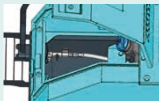
Special sloped crawler side frame design is easily cleaned of mud.
