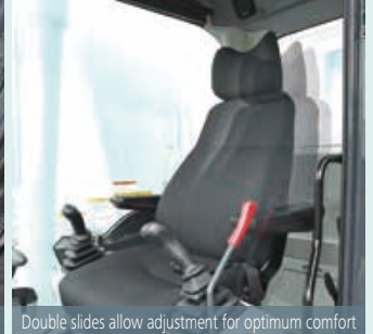
Double slides allow adjustment for optimum comfort
