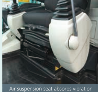
Air suspension seat absorbs vibration
